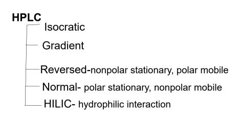
Common column- 100-200 mm long and 3-4.6 mm diameter Smaller diameter offers better separation and sensitivity
